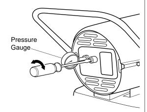
Figure 13 - Adjusting Pump Pressure
